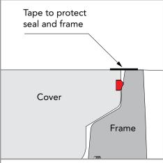
It is recommended that during concreting, the cover be postioned into the frame and the gap between the cover and frame be sealed with tape to protect the cover seal and frame.
