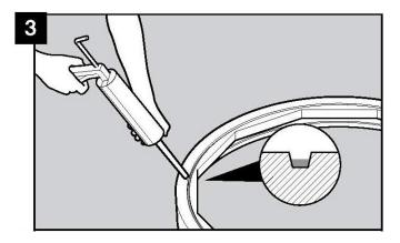
Invert the frame so channel is facing up and apply a continuous bead of adhesive sealant in the frame channel – use Soudaflex, Bostik 1100FS or similar adhesive.
