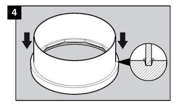
Push the skirt into the frame channel so that it seats into the channel. Only one side of the skirt will fit the channel – the smaller diameter side of the skirt.
