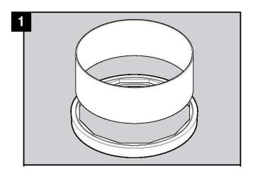
Turn the frame upside down and "dry fit" the skirt into the channel to ensure proper fit. Notify Fibrelite if skirt does not fit properly or another size is needed. Do not bond skirt unless correct.
