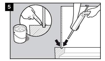
Apply a bead of adhesive sealant to both the inside and outer edge (as shown) and smooth off with wet finger.
