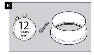
Allow for a minimum 12-hour cure time before proceeding with the frame installation.
