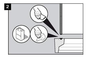
Thoroughly sand the channel and the top edge of the skirt. After sanding, clean both surfaces using acetone to remove any dust or debris that remains in the channel.
