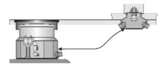
**12.1.2 Between Dispenser Sumps:** For other Access Pipe chase pipe sections running between dispenser sumps measure the distance from one dispenser sump wall to the next allowing for the natural chase pipe position between sumps. Make an allowance in your measurement for the chase pipe to gradually weave side to side within the trench to allow for future thermal expansion and contraction of the flexible supply pipe section contained within.
