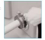
WARNING: Do not over tighten the band clamp beyond the maximum torque of 30 inch pounds or it is possible to damage the rubber boot.
