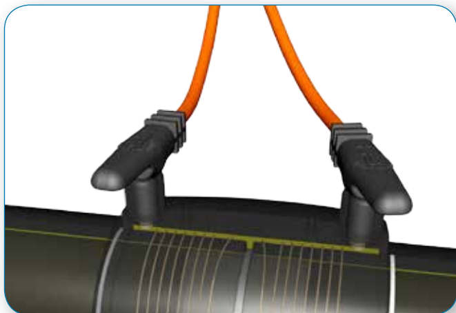
During electrofusion welding material is melted by the heat from the socket wiring and the pipe fuses with the welding socket.
