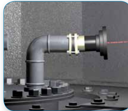
Place the laser pointer in the pre-mounted fittings on the manway lid.
