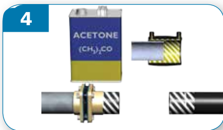
Clean the area on the pipe and transition fitting that will be welded and the inside of the welding socket with acetone or isopropanol.
