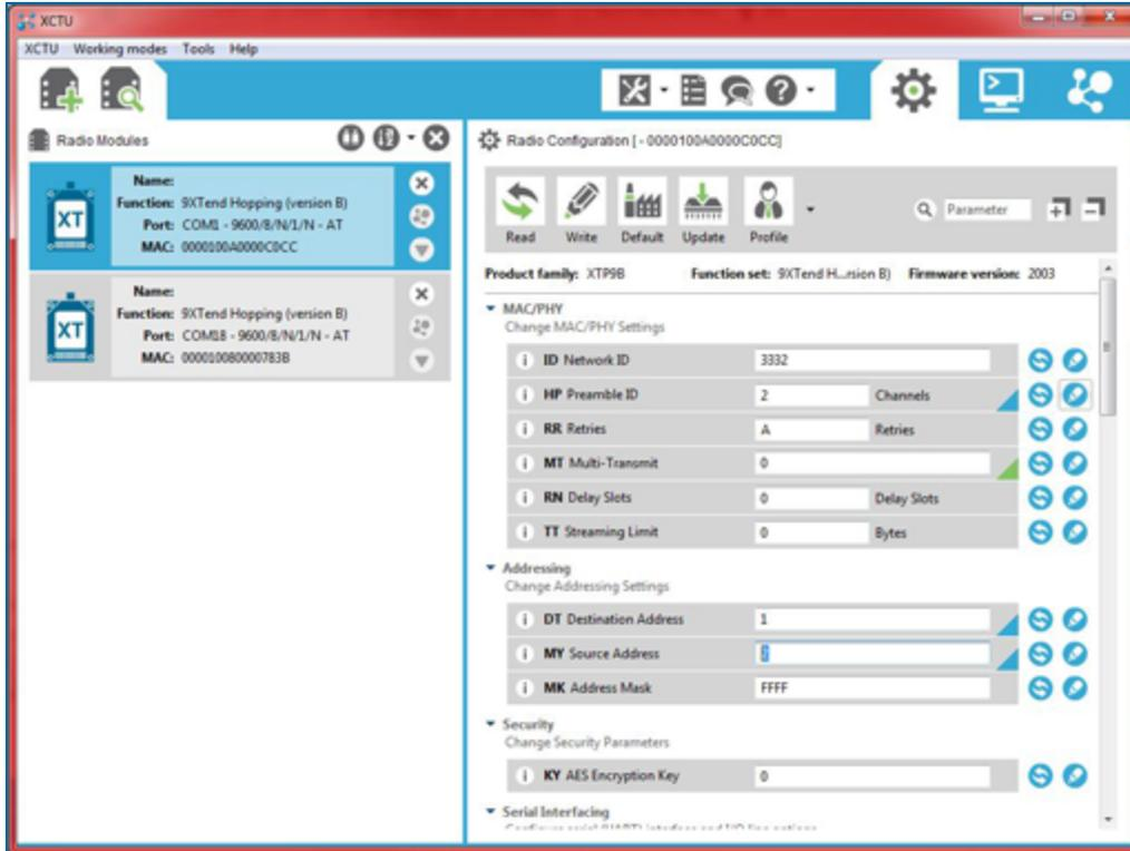
Figure 3-4 Modem #2 Configuration
