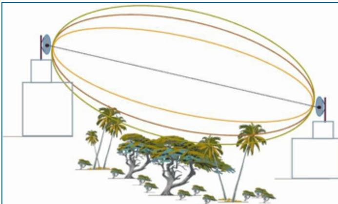
Figure 2-2 Antenna Height Over Physical Obstructions
