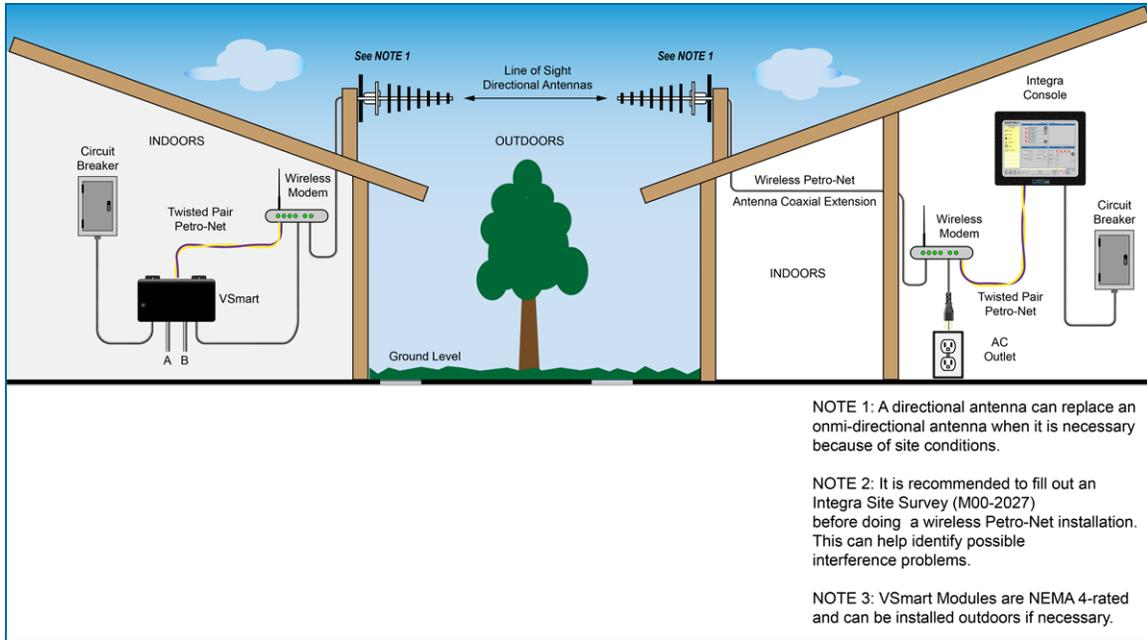
Figure 2-6 Wireless Installation with VSmart Indoors
