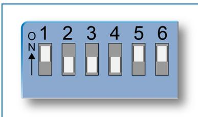
4. Set both Radio DIP switches to RS-232 mode: (Switch #1, #5, #6 up [ON] and the remaining switches are down [OFF]).
