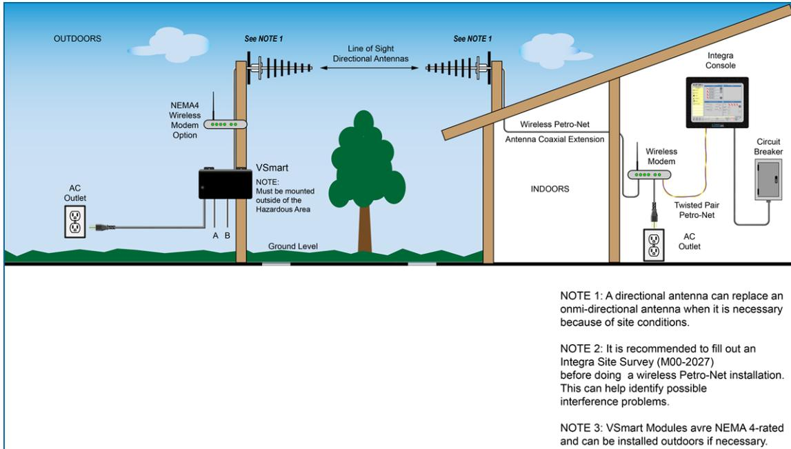
Figure 2-5 Wireless Installation with Outdoor Pole-Mounted VSmart
