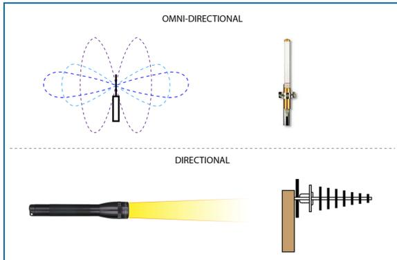
Figure 2-3 Omni-Directional and Directional Antenna Signal Patterns
