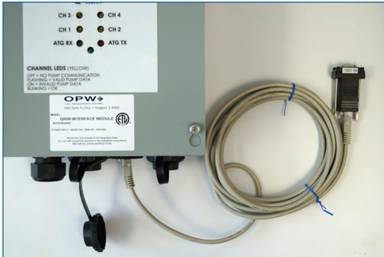
Figure 6-2 Serial Adapter Connection
