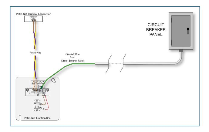
**NOTE:** Petro-Net twisted pair wires can also be black and white. The connections between the terminal and the Petro-Net Junction Box must still maintain the 1 to 1 and 2 to 2 number connections as described above.
