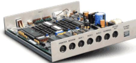
*Figure 1: System2 Fuel Site Controller (FSC)*
