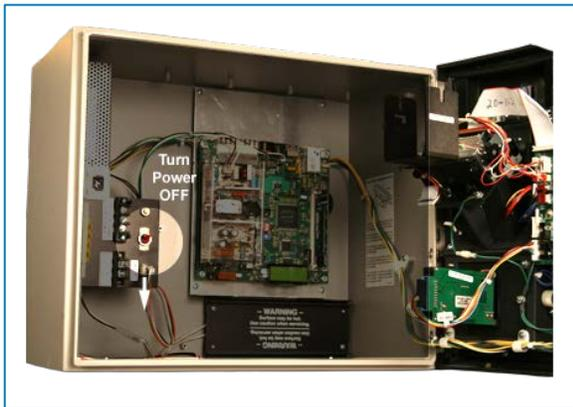
2. The red power supply toggle switch is located on the left rear of the console. Flip the switch down to the OFF position to power down the unit.
