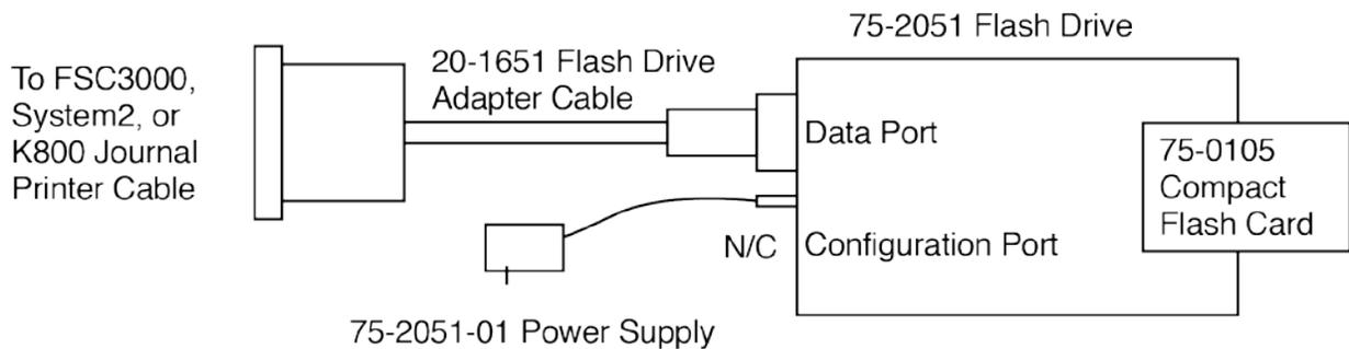
Figure 1-2 Data Recorder Connection Diagram
