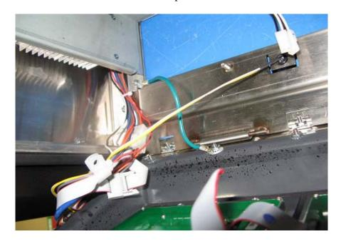
11. Mount door onto hinges, remove the kep nut on the FIT500 enclosure and door. Using the 20-1601 green ground strap, attach to the unit as shown.
