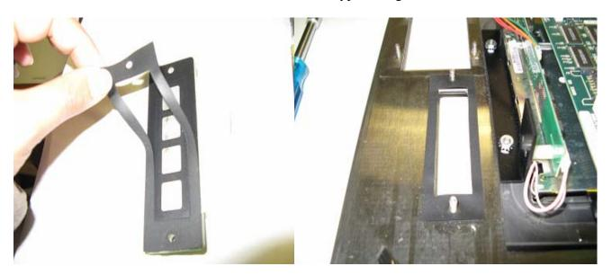
7. Reuse old gasket and place new metal keypad securing with old kep nuts.
