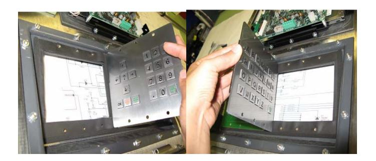
3. Reuse old gasket and screw in new metal keypads as shown, with the provided screws.
