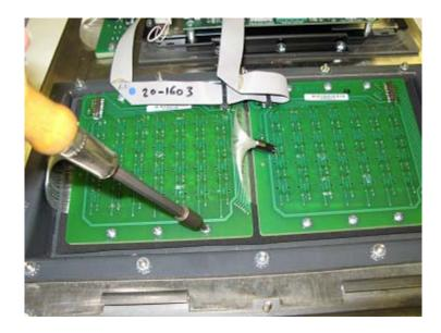
2. Remove and discard the 12 screws holding the keypads in place, new shorter screws have been provided. (If you try to use the old ones you risk puncturing the unit.) Remove and discard keypads.
