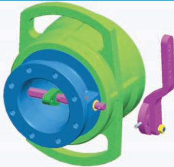
Step 3: Feed poppet through nose seal sub-assembly. Remove cylinder and wave spring.
