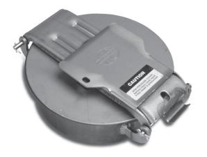
The LA 8" Fill Cover is a low profile, easy opening, positive seal unit. This unit comes with a 3" high standard weld ring, the design and strong steel stamping ensure a long lasting, easily maintained Fill Cover. The LA 8" is available in all steel or stainless contact parts with external plated steel. A Buna-N gasket is standard, but other gasket materials are also available.
