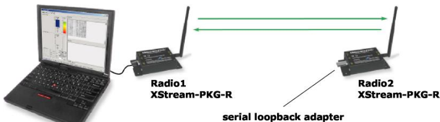
Figure 5-2 Range Test Cable Setup
